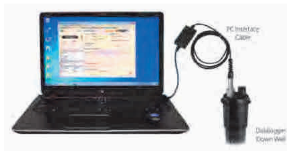
Solinst Levellogger and direct read cable connected to a PC using a PC interface cable
